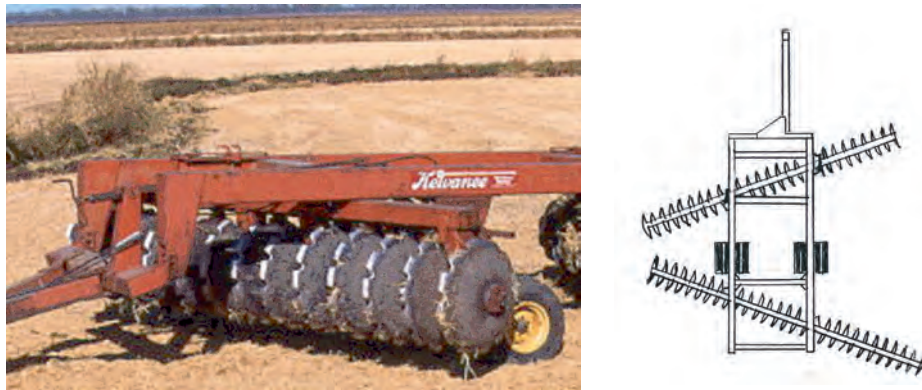
Figure 2. Heavy-duty single offset disc, called a stubble disc, for use in fall straw incorporation (left). Lighter versions with smaller blades are used for spring tillage. On the right, a schematic overview of a typical single offset disc.
